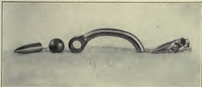
FROM LEFT TO RIGHT: BULLET LODGED IN GASOLINE TANK AT THIRTY- SIX HUNDRED FEET. SHRAPNEL BALL WHICH WENT THROUGH CAR- BURETER AT TWENTY THOUSAND FEET. TAPPET ROD WHICH BURST AT SEVEN THOUSAND FEET. BULLET WHICH STRUCK AUTHOR IN SIDE
